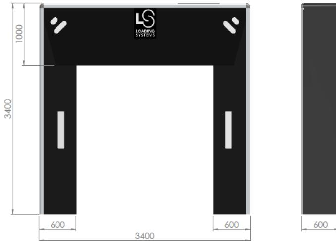
The PowerShelter 403M is a dock shelter which uses a sturdy curtain made from durable material for the closing of the area between the opening of the warehouse and the docked vehicle.
